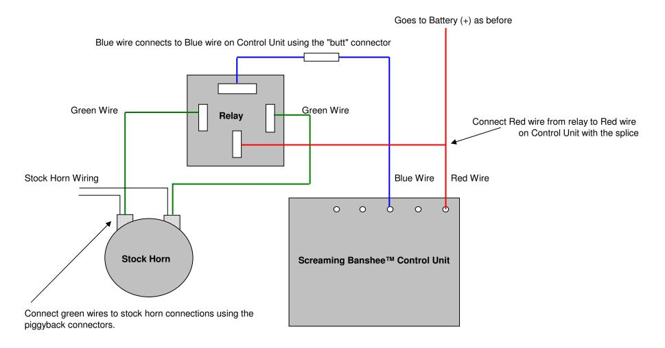
Note: All other wires to the Control Unit are wired as before - no other changes are required
